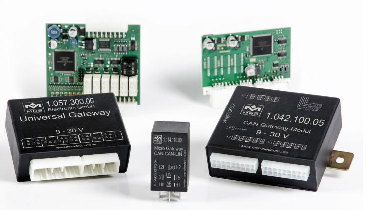
Gateways are the central contact point for all control units. They can transmit and evaluate all information and data, allowing all electronic control units to communicate and work together. They are used primarily in the automotive sector, where they control and coordinate all ECUs in vehicles. This enables error-free, secure communication between all controllers.
